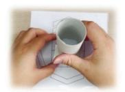
3. When you get the micro:bit from teacher (or you may complete last few steps at the class), put the battery box of micro:bit into the toilet paper tube, and cut a 4-cm long gap to hide the wire; and then stick the micro:bit to the top of the toilet paper tube with a Blu-Tack.
